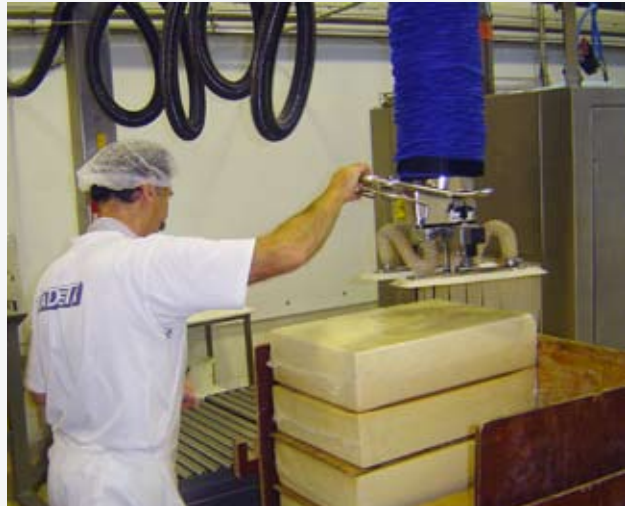
3. A stainless steel VM200 unit is used to lift and package these blocks of cheese in the packaging area. The suction foot used is a standard 620600 with white gaskets.
