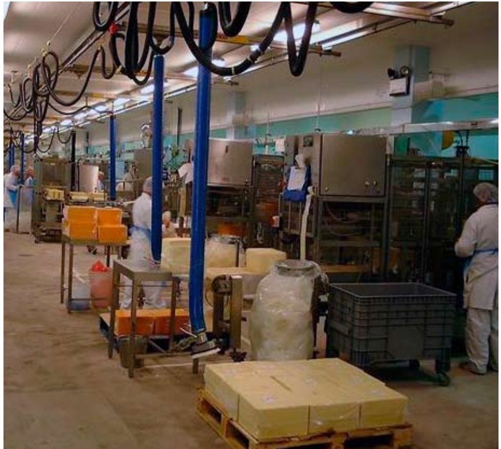
1. Stainless steel units are often requested in the food industry and in pharmaceutical industry. Several stainless steel VM120 units are installed in this cheese manufacturing facility. Photo, left: VacuEasylift can also be used to lift sacks.
