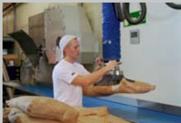
1. Stainless steel units are often requested in the food industry and in pharmaceutical industry. Several stainless steel VM120 units are installed in this cheese manufacturing facility. Photo, left: VacuEasylift can also be used to lift sacks.
