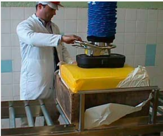
4. A VM160 cheese lifting application for blocks of cheese weighing appr 60-70 kg. Food industry have been using vacuum lifters to handle food stuffs in the cold packaging area for many years.
